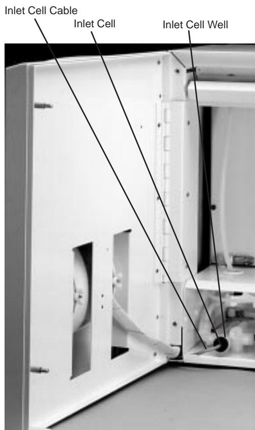
Figure 12 Inlet Cell Installation and Location
